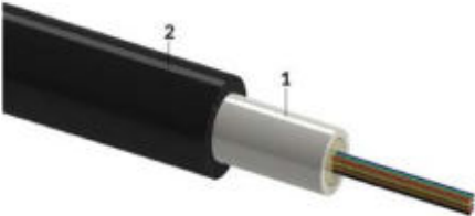
1. Gel filled PBT loose tube with optical fibers 2. UV stable HDPE outer sheath
